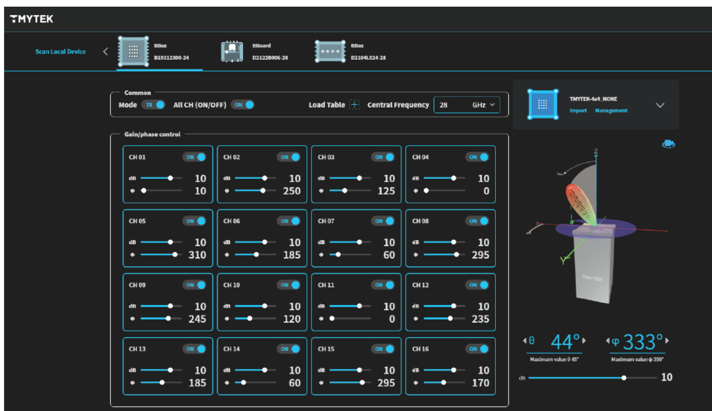
Figure 7: BBox™ One GUI developed by TMYTEK, which allows users to intuitively control the amplitude and phase of each channel.
