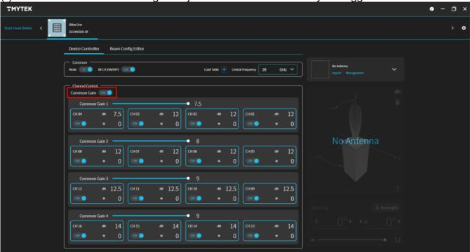
(9). Adjusting the common gain will simultaneously affect the gain of the 4 channels on the board. Take this screenshot as an example, if the common gain is changed to 0, the Channel01 is 4.5 dB, Channel04 is 0 dB. Then, the common gain and channel gain can be adjusted separately.
