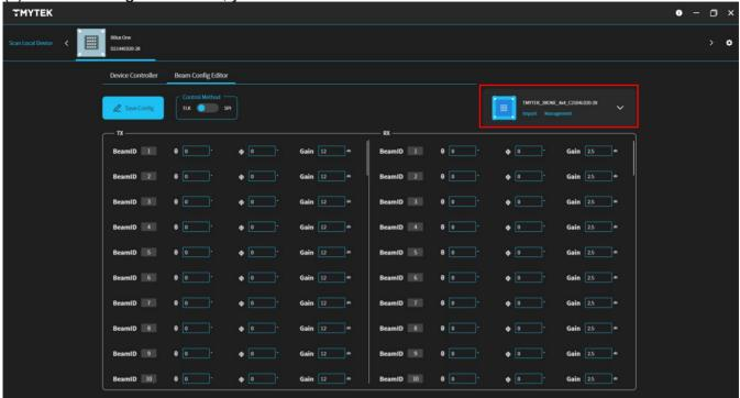
(4).64 sets of beams can be stored in the Tx/Rx mode each, and the range of values that can be entered will be prompted below the input box.
