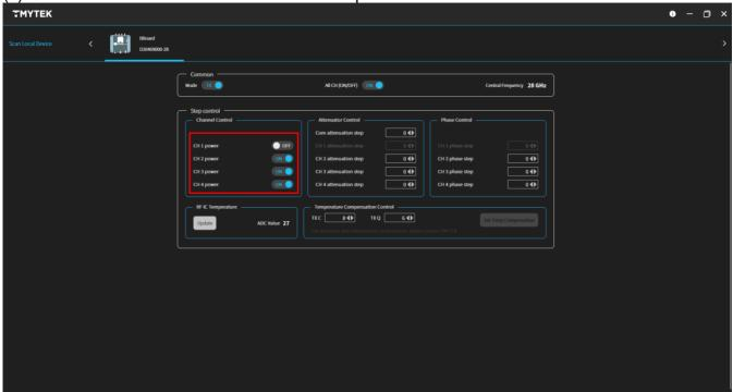
(8). Adjust the Attenuation step to set PA/LNA gain. Step range is 0-15.
