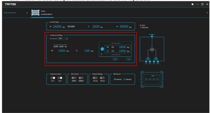
(8). If the input frequency is the same the in-band harmonics, the Current Value will turn yellow and the Harmonic icon in the upper right corner will also turn yellow to signal warning.
