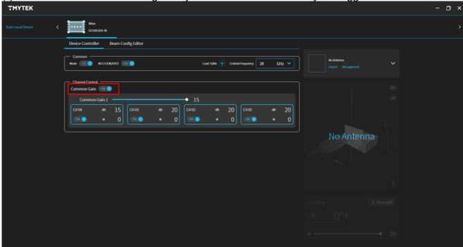
(9). Adjusting the common gain will simultaneously affect the gain of the 4 channels on the board. Take this screenshot as an example, if the common gain is changed to 0, the Channel01 is 5 dB, Channel04 is 0 dB. Then, the common gain and channel gain can be adjusted separately.
