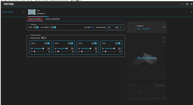
(2). Click the Mode toggle switch to switch between Tx/Rx mode.
