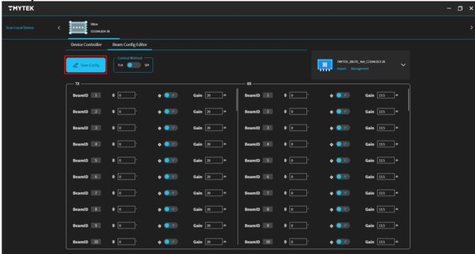
(6). Control Method shows how BBox is controlled. In the "TLK" mode, the device is controlled by Ethernet.
