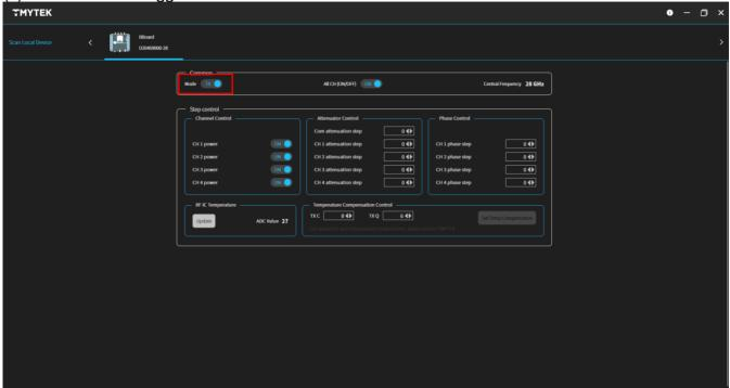
(6). Toggle All CH (ON/OFF) can switch all channels on/off.
