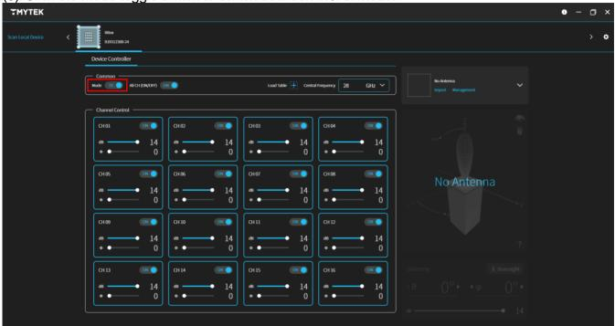
(7). Toggle All CH (ON/OFF) can switch all channels on/off.
