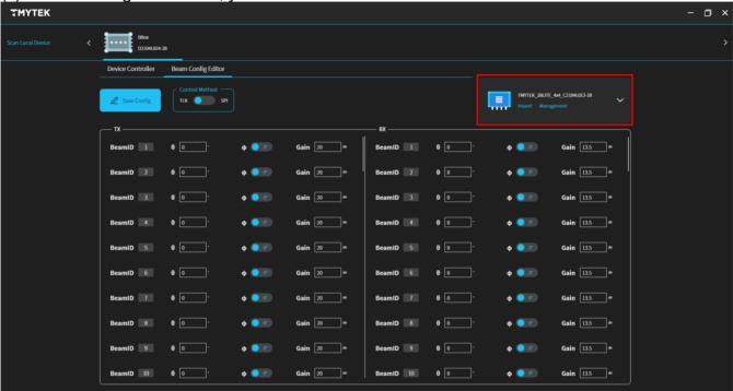
(4).64 sets of beams can be stored in the Tx/Rx mode each, and the range of values that can be entered will be prompted below the input box.
