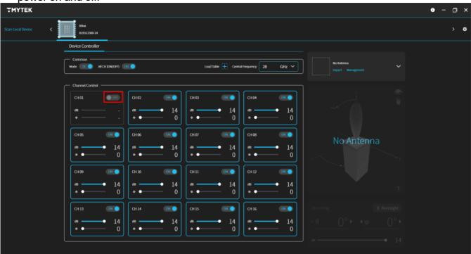
(11). Adjust the sliders of dB and  $\Phi$  in the channel card(s) to control the channel gain and phase.
